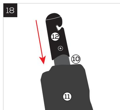
Encase the safety enclosure poles in the PVC sleeves leaving the fixing end for the upper hoop exposed.
