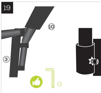
Insert the lower section of the safety enclosure poles into the T-tube connector's and the W foot welded tubes. Then tighten it with the screw using the hex key.
