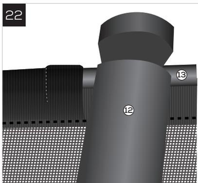
Insert the fiberglass upper hoop inside the fixing end of the safety enclosure poles. Make sure the entrance of the safety net is set between two W feet.
