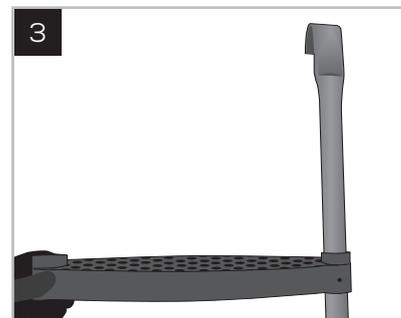
**NOTE:** The plastic step is not flat, position it parallel to the ground.
